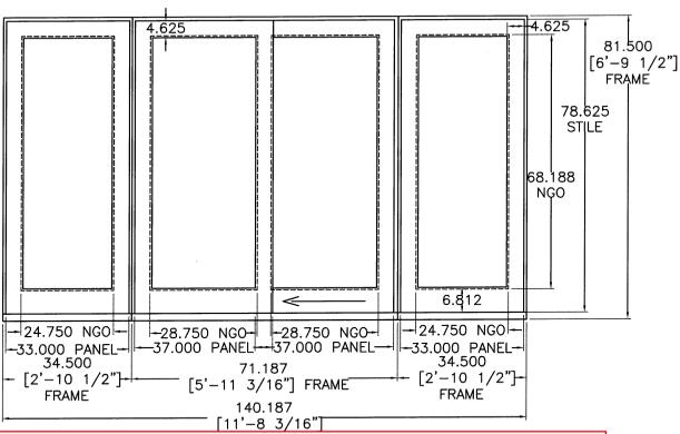
Exterior color and material will match existing sliding glass door. Owner will need to choose which of the center slider panels to be operational (left or right). For example the drawing above shows a right side opening slider door from the inside (arrow on picture). Feel free to look at Sierra Pacific website for similar examples. http://www.sierrapacificwindows.com/patio-sliding-doors.cfm
